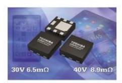
ensures that the MOSFETs achieve low on-resistances. RDS(ON) rating are 6.5mΩ for the 30V SSM6K513NU and 8.9mQ for the 40V SSM6K514NU.
