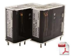
The SGR282ZK has an industry standard footprint and the contact material is silver copper nickel with a gold plate (AgCuNi), its coil voltage range is 5 VDC to 110 VDC.
